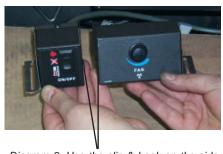
Diagram 3: Use the clip & hook on the side of the control boxes to join them together.
